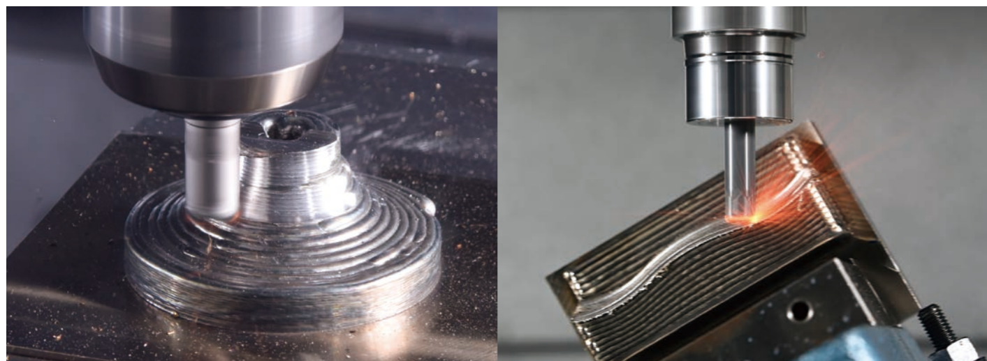
Milling : roughing operations
