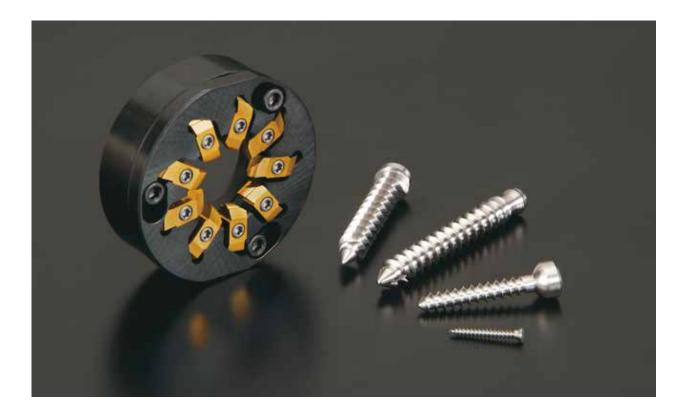
NTK first released thread whirling tools with (9) inserts back in 2008. NTK engineers never perceived thread whirling as a complicated process. The complication was not with regards to machining difficulty but in producing the perfect thread form described on the print itself.
