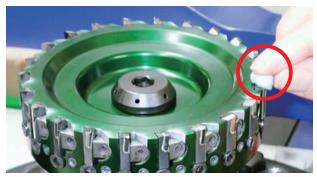
Clean up insert edges using clay.
