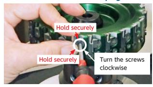
Install the insert to cutter pocket. Tighten wedge set screw with 1Nm torque while pushing insert to cutter center using two fingers. (do not overtighten)
