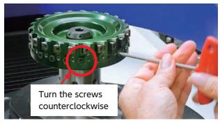
Loosen axial set screw until the screw head is 1 to 2 mm from cutter body. Clean up insert pocket using air.
