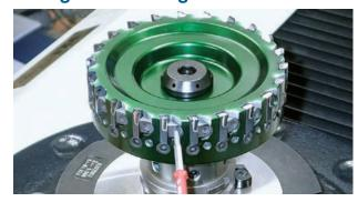
Tighten wedge set screws with 4Nm torque.
