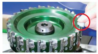
Clean up insert edges using clay.
