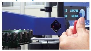
Tighten axial set screws to get 45.000 mm height dimension. Adjust other inserts within +/- 0.002 mm range.
