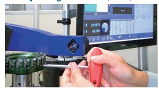
Tighten axial set screw of each insert until you reach around 44.980 mm height dimension.
